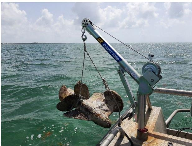
*DEP staff use specialized equipment to aid in the removal of large marine debris, including this boat-engine lower unit removed from Newfound Harbor Patch Reef.*
