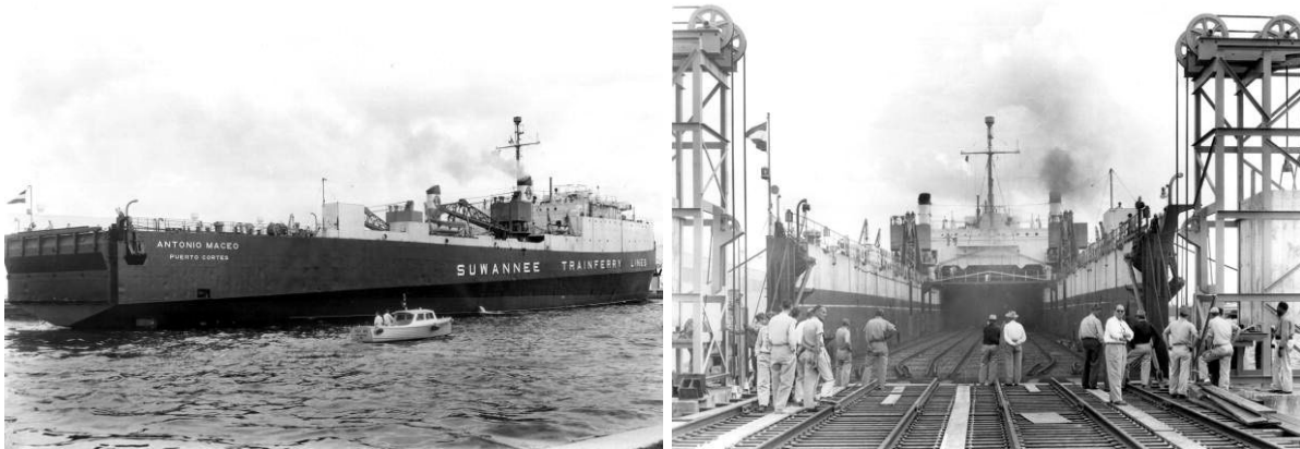
Photo 5: The docking and cargo loading of the Antonia Maceo at Port Everglades in 1953. This vessel was a Cuban car ferry loaded directly from the railroad lines (Photo: State Archives of Florida).
