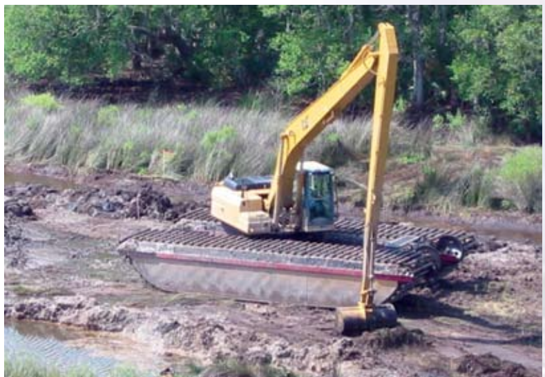
Volusia County Mosquito Control operates an amphibious bucket loader at work restoring impacted wetlands to natural marsh elevations.
