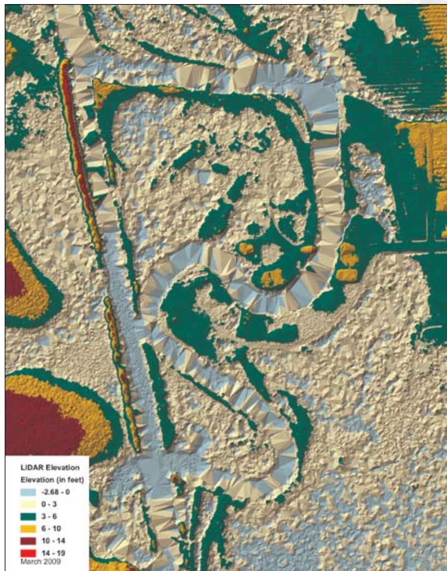
Figure 5 / Light Detection and Ranging (LiDAR) data are used to identify hydrologic restoration areas along the North Fork St. Lucie River and its headwaters. (Data provided by SFWMD.)
